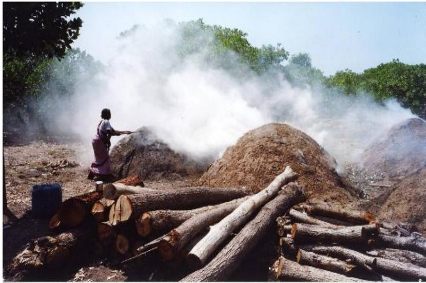
**Figure 25.** Earth kilns built in place (source: <http://www.biocoal.org/10.html>; date accessed: Nov., 15, 2010).
