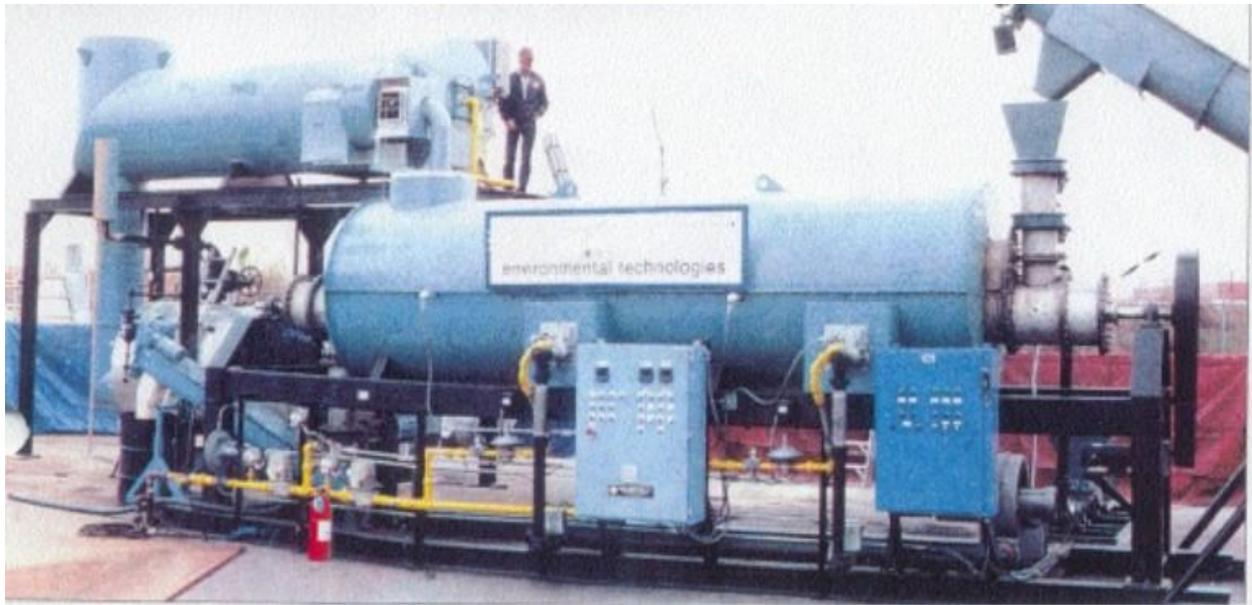
**Figure 68.** International Tech Corporation pyrolysis unit with heat recovery (<http://www.internationaltechcorp.org/IT-info.htm>, date accessed: Nov. 13, 2010).
