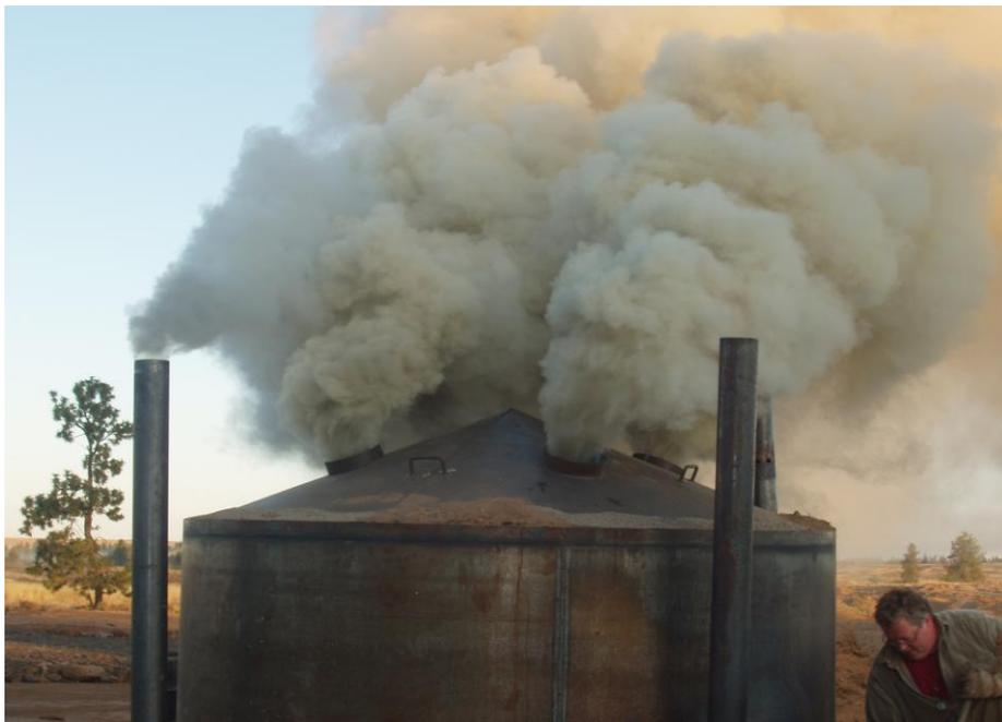
**Figure 2.** Environmental impact of carbonization units without recovery of volatile products (Courtesy of the Washington State Department of Ecology).
