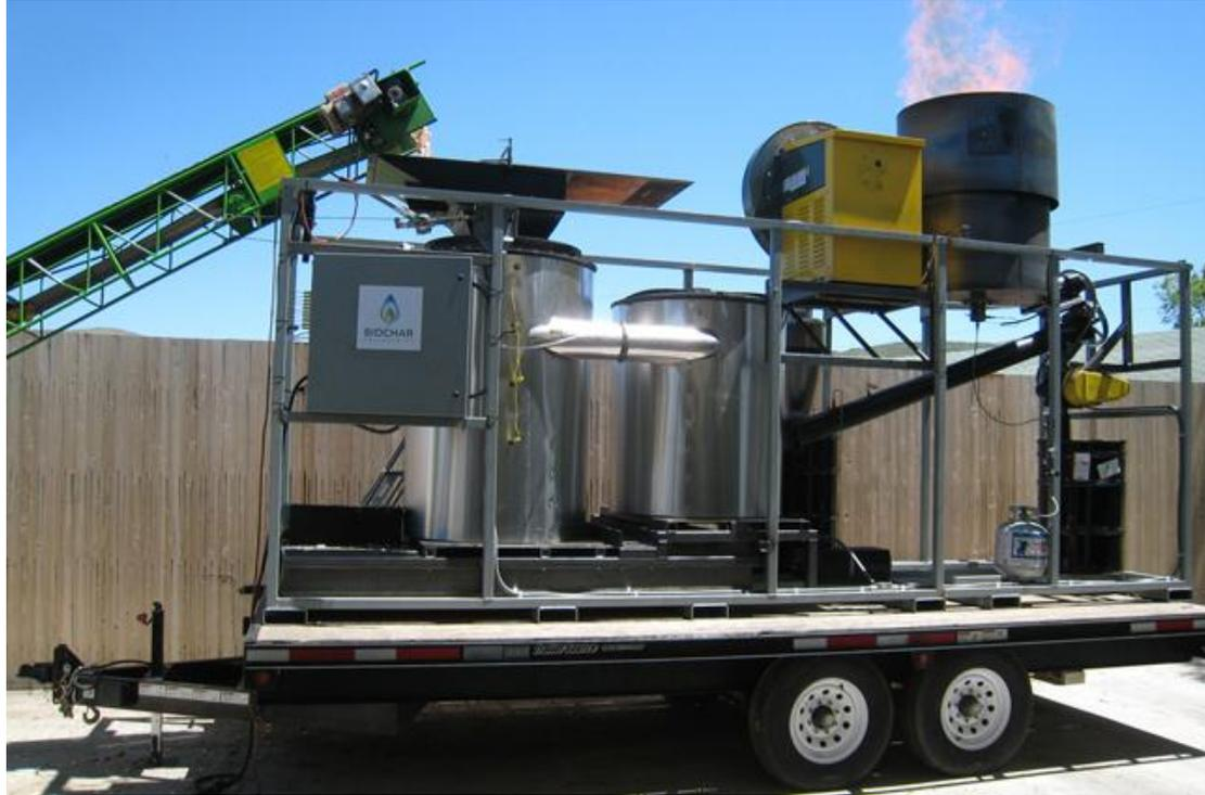
**Figure 58.** Picture of the mobile downdraft gasifier to produce biochar and heat from wood chips (source: <http://www.biocharengineering.com/technology/>, date accessed: Nov. 13, 2010).
