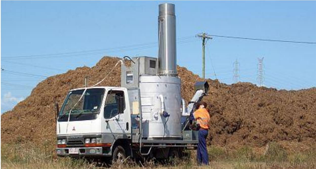
**Figure 60.** Mobile multiple-hearthfurnace commercialized by Black is Green Pty Ltd (<http://www.bigchar.com.au/about.html>, date accessed: Nov. 13, 2010).
