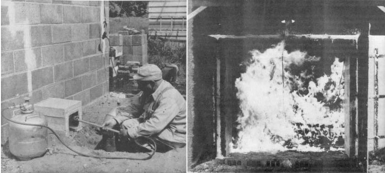
**Figure 30.** Igniting the kiln charge with a gas torch (left); and ignition of the charge by the open door method in an auto-thermal process (right) (Toole et al., 1961).
